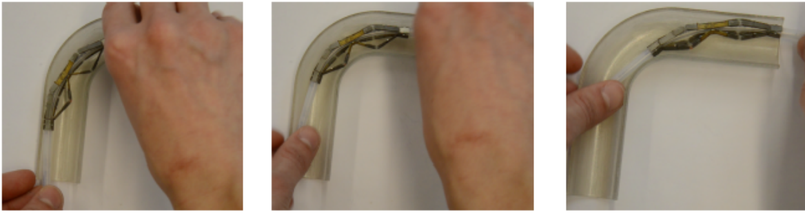
Figure 7.14: Braced catheter turning through the IVC analog.
