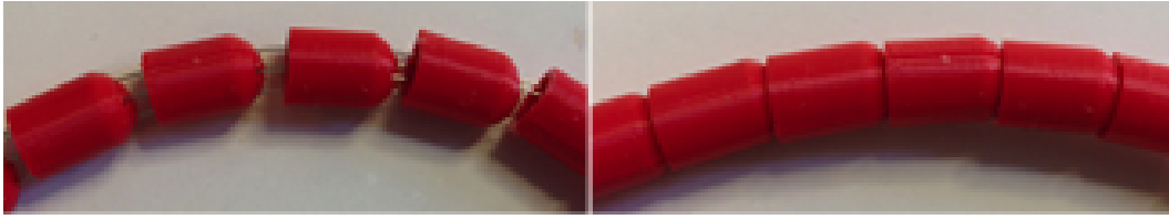
Figure 6.2: (left) Vertebrae are connected in series by pull wires. (right) Pull wires are tensioned to lock vertebrae in place.
