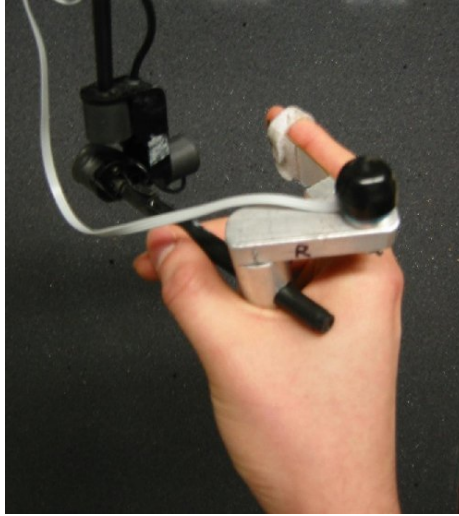
Figure 6.2: Handle addition to Phantom haptic interface
