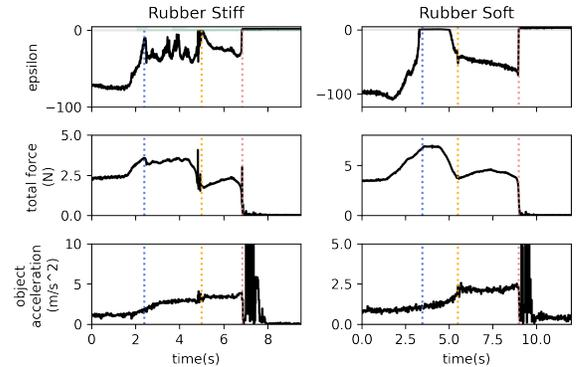
Fig. 3. Grasp analysis results for the rubber cases. Epsilon is a metric of grasp stability that goes to zero at the onset of object slip [1]. The blue, yellow, red lines are when the object first starts to slip, the first finger loses contact, and the object completely drops out of the robot hand, respectively.
