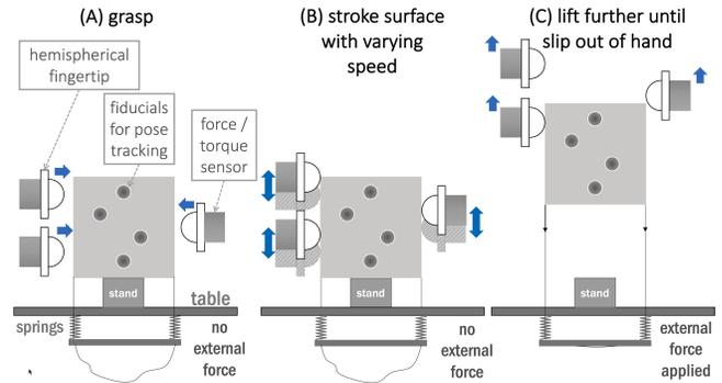
Fig. 1. (A) Components of the system. (B) The stroking experiment: each finger touches the object, sliding up and down in a repeated motion. (C) The grasp-lift-slip experiment: the object is grasped then slowly lifted until external force is applied via a string looped under the table, causing the object to slowly slip out of the robot hand.
