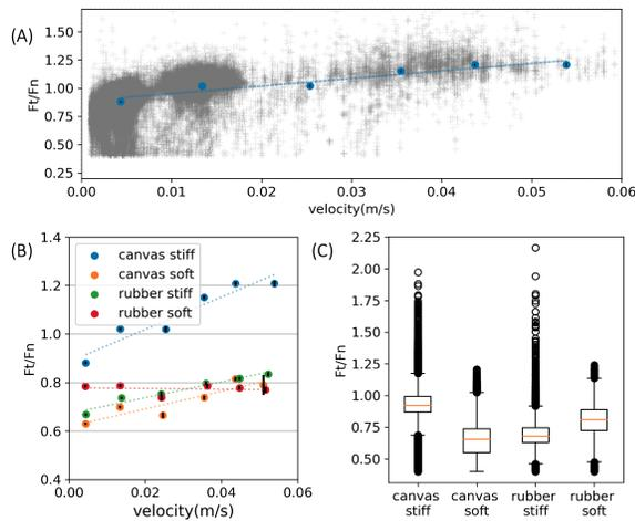
Fig. 2. (A) Typical distribution of coefficient of friction (ratio of tangential to normal force during sliding) versus sliding velocity (canvas stiff case). (B) Trends of coefficient of friction with respect to contact velocity for the four object cases. (C) Soft cases have far fewer outliers and a wider distribution.
