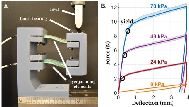
Fig. 2. Experimental characterization of a jamming-based parallel flexure mechanism. **A.** Experimental Setup. **B.** Force-displacement results. Lines represent means at each deflection and the shaded bars are the standard error across trials and samples.
