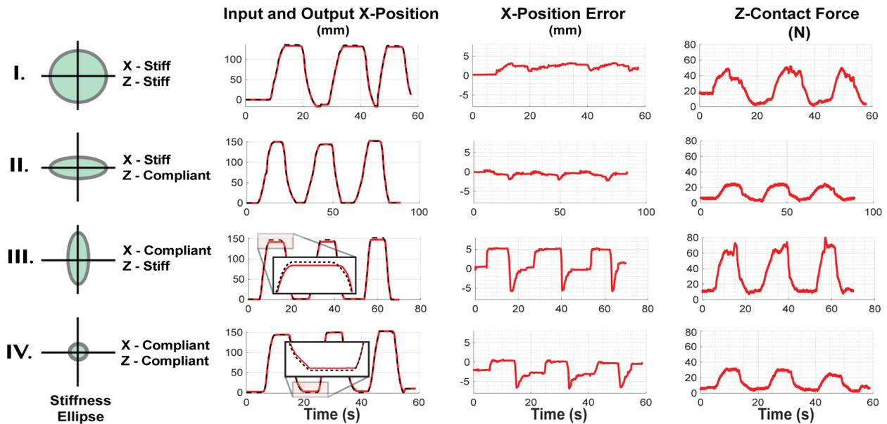
Fig. 4. Position and force data from the tracing task using the jamming-based flexure wrist. The experiment is conducted in four different conditions: **I.** Both axes stiffened; **II.** Only X-axis stiffened; **III.** Only Z-axis stiffened and **IV.** Both axes compliant. The dashed black line is the position input from the robot arm.
