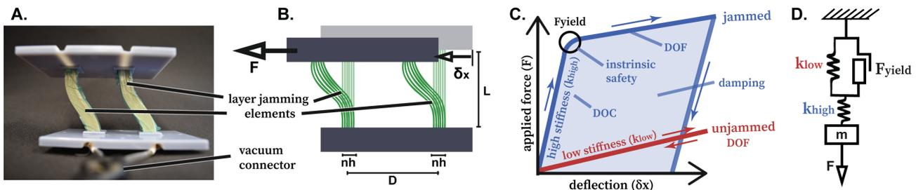
Fig. 1. Jamming-based flexure mechanism. **A.** Physical prototype. **B.** Diagram showing relevant parameters. **C.** Force-deflection plot characterizing mechanical behavior under jammed and unjammed conditions, showing Degrees of Freedom (D.O.F.) where low stiffness allows motion and Degrees of Constraint (D.O.C.) where high stiffness limits motion. **D.** Lumped parameter model of layer jamming structure that captures static and dynamic behavior.
