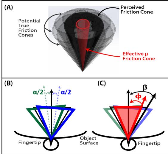
Fig. 5: (A) Perceived, actual, and effective friction cones in 3D. (B) The cross-section of (A), where uncertainty in contact normal results in a range of potential friction cones, bounded by the green and blue cones. (C) the overlap between the green and blue cones, shown in red, is the cone containing the force vectors that can be reliably exerted at the given point; the angle that spans this “effective friction cone” can be calculated by  $\phi = \beta - \alpha/2$ .
