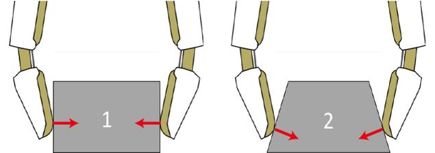
Fig. 1: Robot hand using two-fingered pinch grasp. With a moderate coefficient of friction objects 1 and 2 can both be stably grasped. If, however, the contact sensors in the robot fingertip lack sufficient resolution, then the surface normal direction for object 2 may be so uncertain that grasp stability cannot be reliably predicted.
