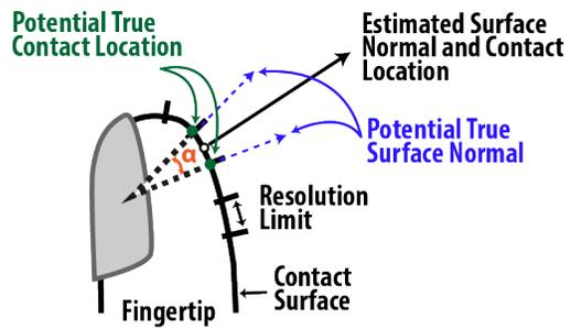
Fig. 4: The sensor resolution is described by a segment of an active area that extends over angle  $\alpha$ , where contacts on the arc covered by  $\alpha$  cannot be differentiated. The actual contact surface normal can differ from the estimated normal vector by as much as  $\alpha/2$ , and the contact location can vary up to half of the length of the receptive field.
