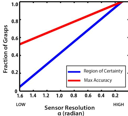
Fig. 11: Implication for Machine Learning. Spatial resolution limits lead to a fraction of the training data being ambiguous, which sets the ceiling for maximum accuracy if those signals are used to train a grasp prediction algorithm. Example here is for spherical objects.
