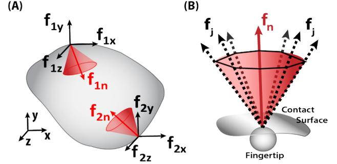
Fig. 3: (A) The point-contact-with-friction model for grasp quality estimation. The force that can be exerted without slipping by each contact is contained within a friction cone. (B) Friction cone is defined by the normal force vector  $f_n$  and coefficient of friction  $\mu$ , but can be approximated by a polygon defined by convex combinations of vectors  $f_j$ .
