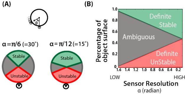
Fig. 8: (A) The placement of the second finger that produces stable, unstable, and ambiguous regions on the circle, (B) As the resolution increases, the size of regraspable region (definitely unstable+ambiguous) decreases.
