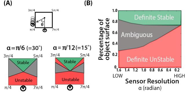
Fig. 10: (A) The grasp is only definitely stable when the fingers are on opposite sides of the square, (B) As the resolution increases, the size of definite stable region increases, the size of definite stable region remains stable, and the size of ambiguous regions reduces.
