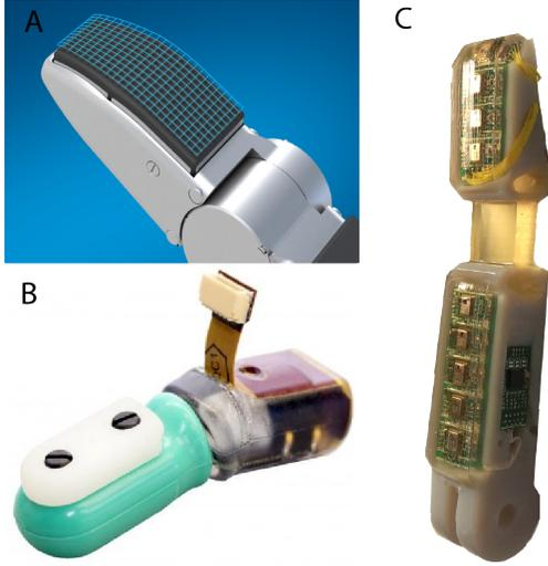
Fig. 2: Examples of integrated tactile sensors on robotic fingers. (A) Tactile array for the Schunk Hand [3], (B) Conductive fluid-filled multimodal fingertip sensor [4] (C) Barometer-based tactile array on a Reflex Hand finger [5].
