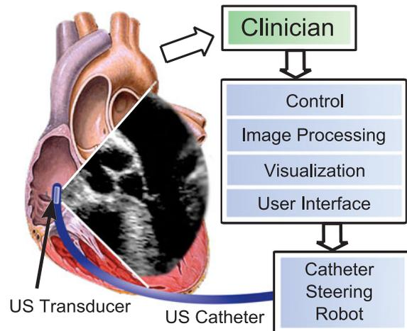
Fig. 1. Diagram of system pointing US imager in the heart.
