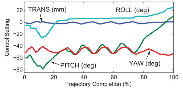
Fig. 17. Actual joint adjustments required to rotate the US imager while remaining at a fixed location.
