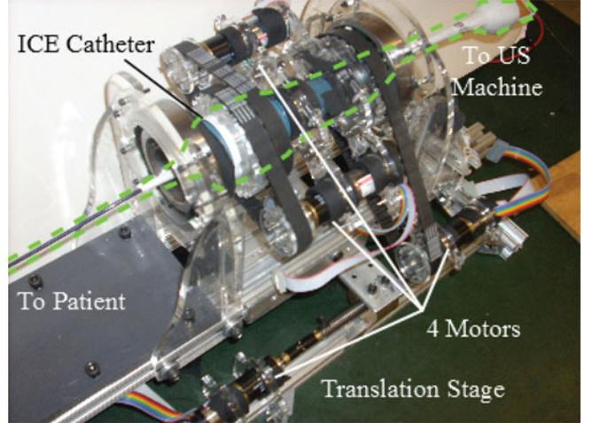
Fig. 11. US catheter steering robot with 4-DOF.—Dashed outline shows catheter handle location within control actuators.
