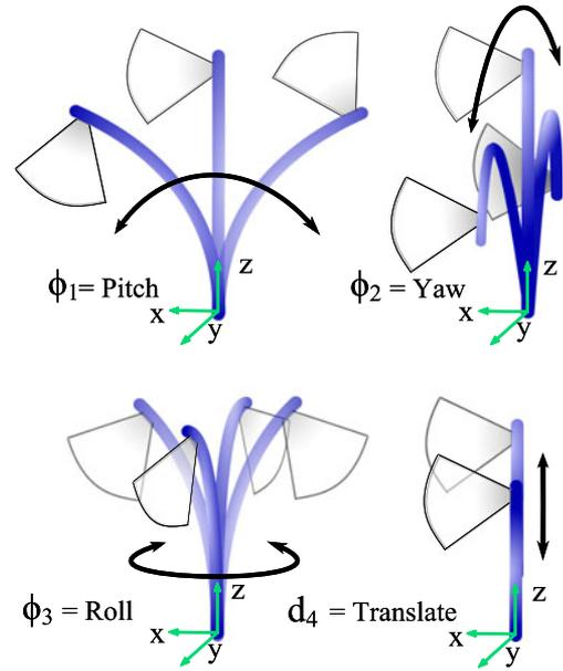
Fig. 3. Corresponding tip motion directions.
