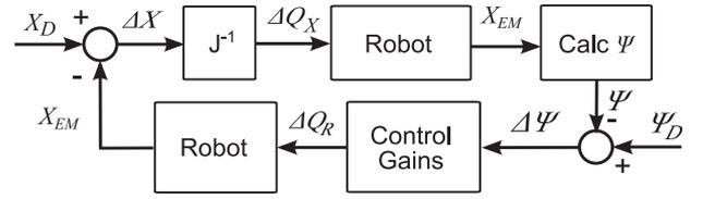
Fig. 13. Control diagram for position and imaging angle.
