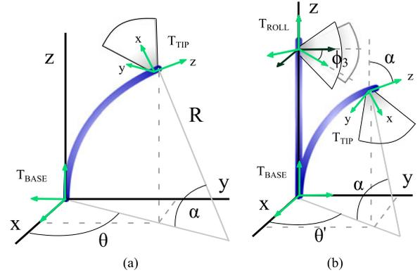
Fig. 5. (a) Catheter bending geometry, (b) inverse kinematics.
