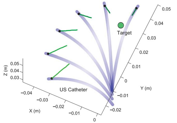
Fig. 20. Results of 3-D pointing tests (green vectors represent the imaging plane pointing at the target).
