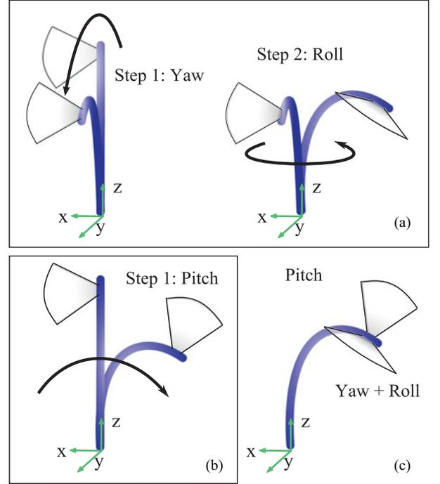
Fig. 6. (a) Yaw and roll are applied to the catheter. (b) Pitch is applied to the catheter. (c) Two cases are overlaid demonstrating that the catheter may be position controlled to the same location with varying orientations.
