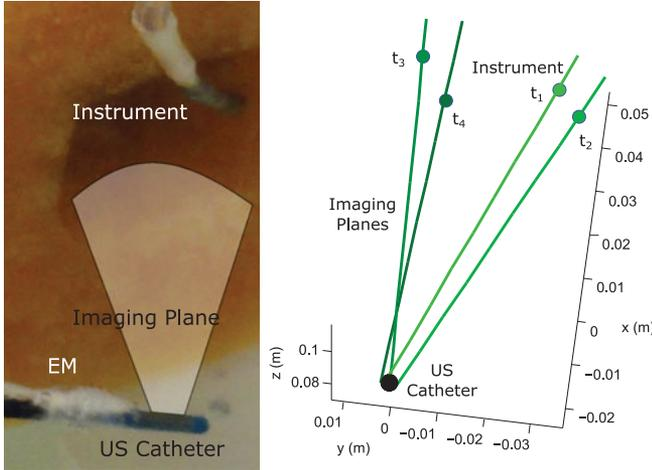
Fig. 18. (top) Photo of tracking the instrument tip and example results from four trials. Lines show imaging plane vectors intersecting ablation tooltip positions represented by circles. Targets are within  $\pm 1$  mm of the imaging plane centerline, thus appearing in the images. (bottom) Additional instrument tracking results based on EM-reported angle errors.
