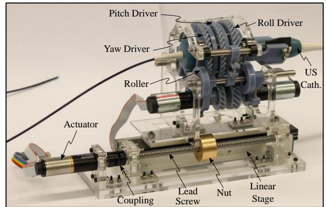
**Figure 7: FULLY ASSEMBLED ROBOTIC SYSTEM**
