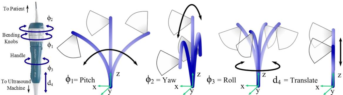
**Figure 1: CATHETER HANDLE DEGREES OF FREEDOM AND RESULTING CATHETER TIP MOTIONS**
