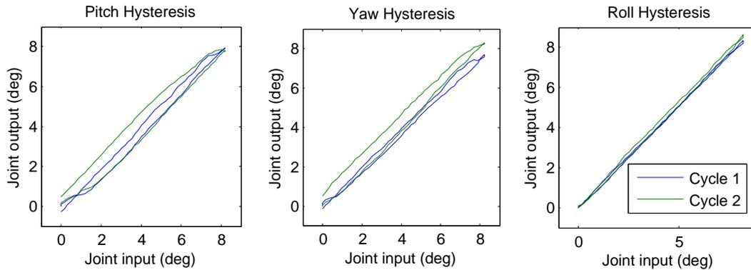
**Figure 10: HYSTERESIS CURVES FOR ROTATIONAL JOINTS**
