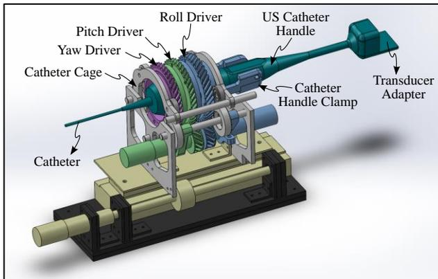
**Figure 6: CAD MODEL OF THE COMPLETE ROBOTIC SYSTEM**
