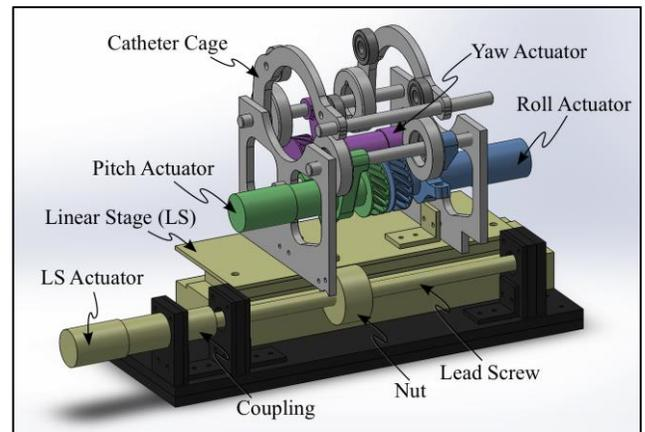
**Figure 5: CAD MODEL SHOWING ACTUATOR ARRANGEMENT**
