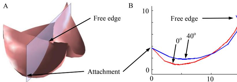
Fig. 3 (A) Simulation result showing mesh of loaded valve with cut plane through leaflet midline. (B) Leaflet midline for right coronary cusp for collagen bundle angle of 0° (red) and 40° (blue). Axis labels are in mm.
