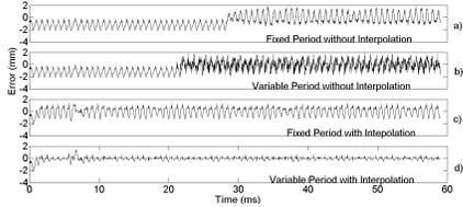
Fig. 8: A comparison of the error when ZOH interpolation a) and b) or cubic interpolation c) and d) is used and when the estimated heart beat length is updated b) and d) or not updated a) and c).
