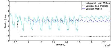
Fig. 10: The motion of the surgical tool tip and the corresponding distance between the simulated heart and the tool tip when no Smith predictor or estimated heart motion is used.
