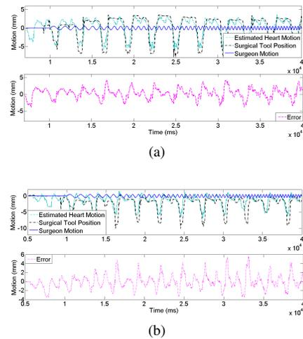
Fig. 11: The motion of the surgical tool tip and the corresponding distance between the simulated heart and the tool tip when (a) cubic interpolation and (b) ZOH interpolation is used.
