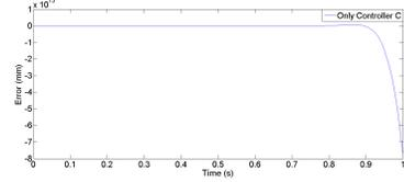
Fig. 6: The distance between the heart wall and the surgical instrument's tip when only a PID controller is used and the delay is present in the system. This case has unacceptable performance as the distance between the surgical tool and the heart wall continually increases.
