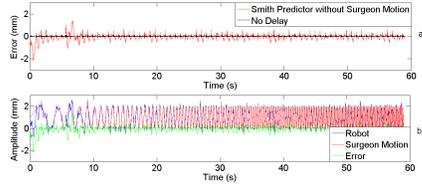
Fig. 7: The distance between the heart wall and the robot end effector when the surgeon’s motion is removed (a) and when it follows a chirp signal with a frequency ranging between 0.1 Hz and 2 Hz with an amplitude of 2 mm (b).
