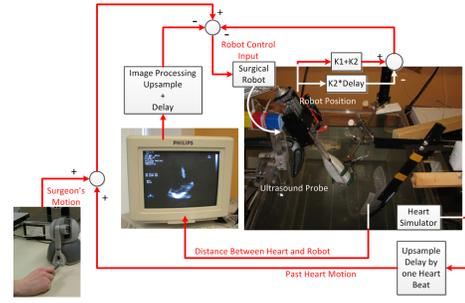
Fig. 9: The experimental setup. A linear voice coil motor actuates a needle which follows the heart simulator based on ultrasound guidance.
