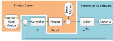
Fig. 3: The initial representation of the feedback controller that controls the robot's motion to follow the surgeon's motion.
