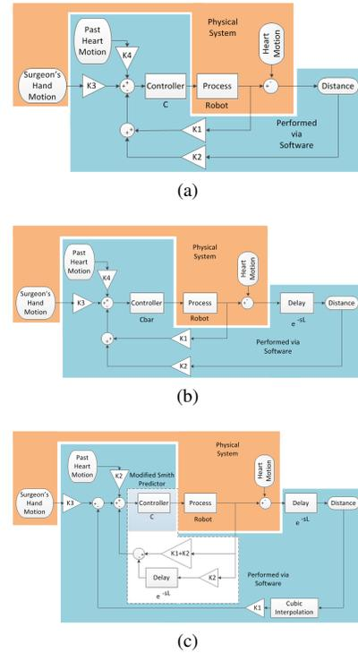
Fig. 4: The feedback controller designed to follow the surgeon's motion as well as the heart's motion with the added gain blocks, which increase the number of design parameters, is shown in a). The initial controller is then replaced by a Smith predictor in b). The complete control loop including the Smith predictor is shown in c).
