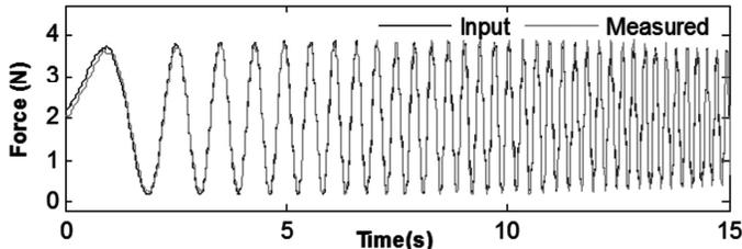
Fig. 5: Input force and sensor response for linear force chirp from 0 to 6 Hz
