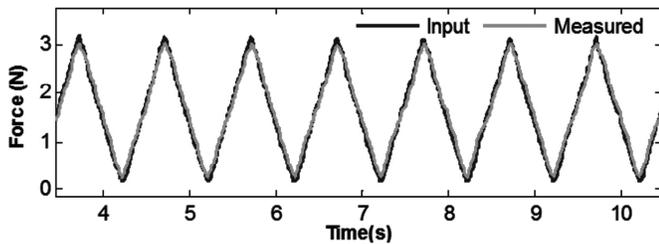
Fig. 6: Triangle wave force trajectory (measured force vs. applied force).
