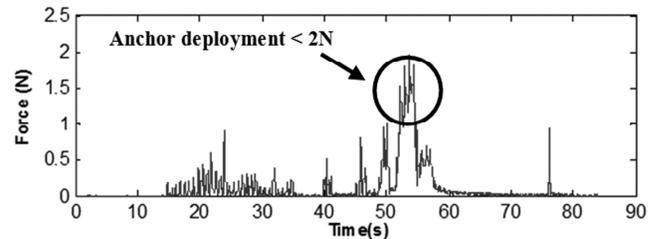
Fig. 9: Anchor deployment forces.
