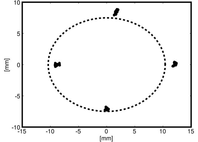
Fig. 9. The instrument was commanded to move to 4 locations. The plot shows the final tip positions for the four commanded locations as circles. The dotted circle indicates desired location.
