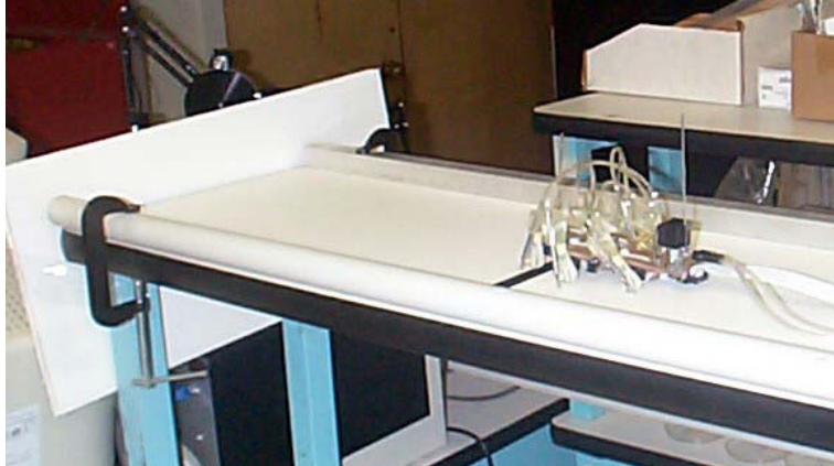
Figure 11: The racetrack. Sprawlita is positioned at the 0.5 meter mark and will run until she hits the wall at the end. Guard rails were placed on both sides to help prevent injury in the event of a wild run.
