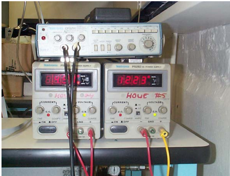
Figure 10: Power sources supplying the pneumatic valves (5V) and the leg servos (12V). The function generator on top provides the alternating square wave fed to the valves, which engage the alternating tripod
