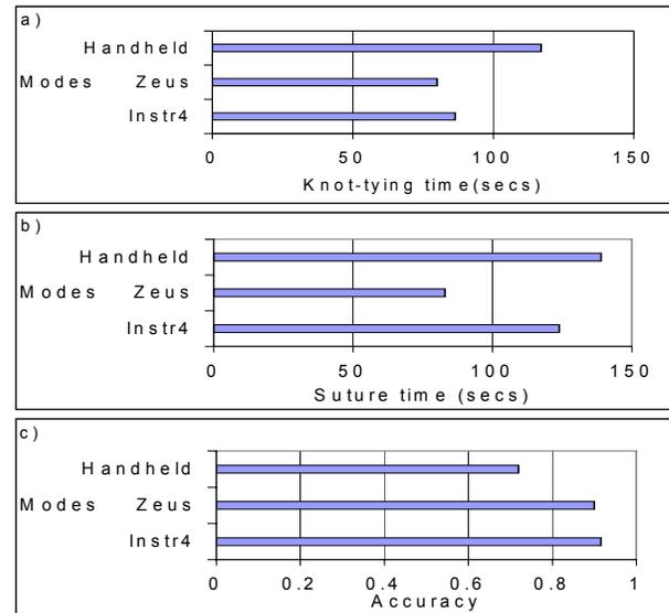
**Figure 8.** Comparison with trained surgeons using handheld instruments and complete Zeus system: (a) knot-tying time, (b) suture time, (c) accuracy
