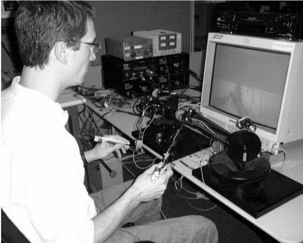
**Figure 2.** Phantoms as master controllers with 6DOF interface. The 4DOF interface is implemented by extending the stylus backwards through a constraint.
