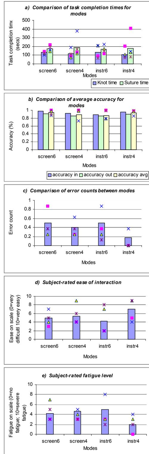
**Figure 6.** Comparison of the 4 modes by performance measures: (a) knot-tying and suture time, (b) accuracy, (c) error count, (d) interface rating, (e) fatigue rating. Symbols show subject averages.
