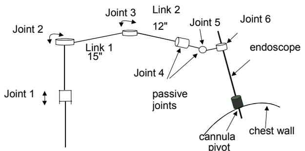
**Figure 1.** Above: block diagram showing Zeus system components. Below: Zeus positioner robot link diagram. Endoscopic robot shown; instrument robots are similar.
