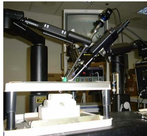
**Figure 5.** Zeus slave configuration: two instrument positioners and one endoscopic positioner inserted into an endoscopic trainer box.
