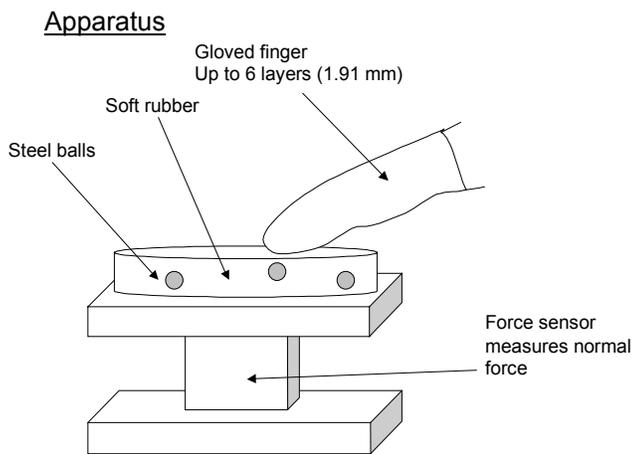
**Figure 1. Experimental setup for the lump detection test**
