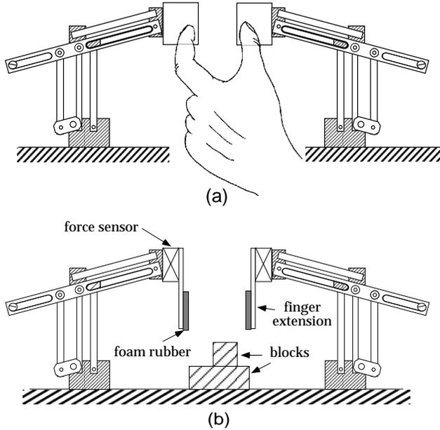
Figure 4: (a) Master manipulator with operator’s hand. (b) Remote manipulator.
