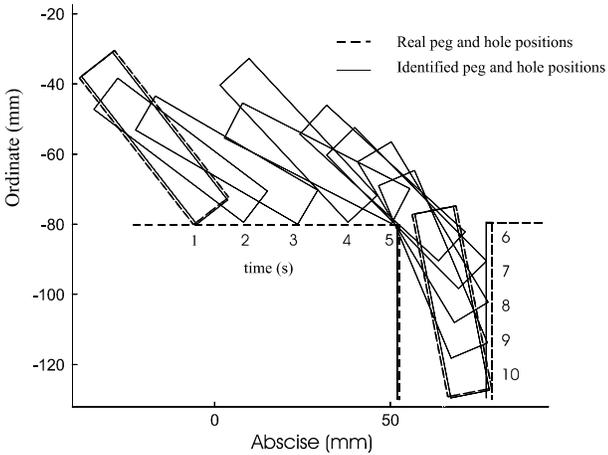
**FIG. 4.** Actual and estimated peg and hole locations. The peg is depicted at one second intervals during the insertion task.
