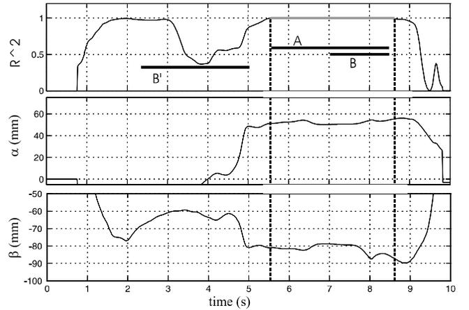
**FIG. 6.** Segmentation of subtask 3, “1-contact peg insertion”. Contact state is A. See (10). Hatched segment obtained using correlation coefficient. Solid segment corresponds to manual operator segmentation by switch.
