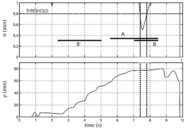
**FIG. 7.** Segmentation of subtask 4, “2-contact peg insertion”. Contact state is {A,B}. Hatched segment denotes where standard deviation,  $\sigma$ , of (17) indicates contact B is active. Solid segment marks manual operator segmentation by switch.
