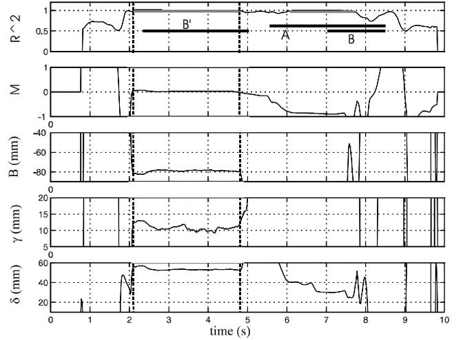
**FIG. 5.** Segmentation of subtask 2, “Slide toward hole”. Contact state is B’ corresponding to (11). Hatched segment obtained using correlation coefficient. Solid segment corresponds to manual operator segmentation by switch.
