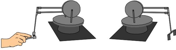
**FIG. 1.** Two PHANToM® haptic devices used as a teleoperator system.
